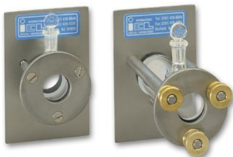
Figure 18: Sodium chloride solution cell. Image reproduced with permission from International Crystal Laboratories (Garfield, NJ, USA).
